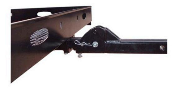
Step.2 Insert four 3/8"x7/8" bolts on the bottom of your carrier tube. Tighten bolts firm with a wrench. See the figure.
