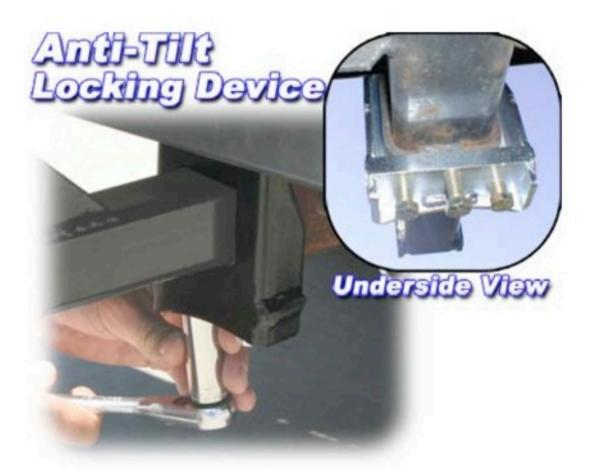
Next loosen the bolts on the anti-tilt lock bracket. (There should be grooves where the bolts were tightened against the hitch receiver)
